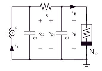
Figure 1: Chua's circuit consists of a linear inductor L, a linear resistor R, two linear capacitors  $C_1$  and  $C_2$ , and a nonlinear resistor  $N_R$ .
