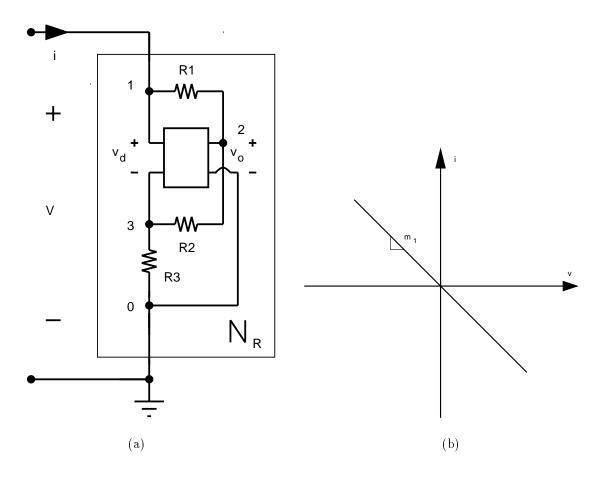
Figure 5: (a) Negative resistance convertor using a voltage-controlled voltage source; (b) v-i characteristic of negative resistance convertor using a linear VCVS with linear voltage transfer function  $v_o = Av_d$ . The slope of the v-i characteristic is given by  $m_1 = \left[\frac{(1-A)R_2 + R_3}{R_1[R_2 + (1+A)R_3]}\right]$ ; for sufficiently large  $A, i \approx -\frac{R_2}{R_1R_3}v$ .
