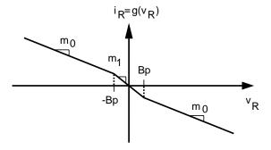
Figure 2: Three-segment piecewise-linear v-i characteristic of the nonlinear resistor in Chua's circuit. The outer regions have slopes  $m_0$ ; the inner region has slope  $m_1$ . There are two breakpoints at  $\pm B_P$ .
