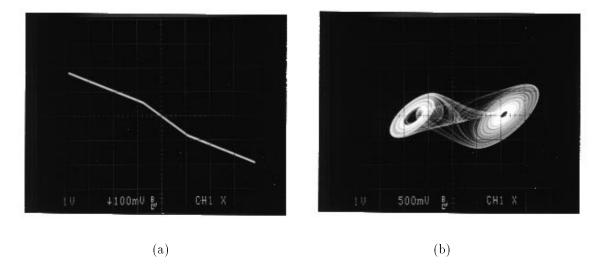
Figure 18: Asymmetry induced by unequal positive and negative op amp saturation levels. (a) left breakpoint of the v-i characteristic is smaller (in magnitude); (b) attractor is asymmetric.
