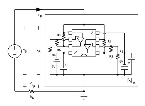
Figure 12: The v-i characteristic of negative resistor  $N_R$  can be measured by applying a triangular voltage waveform  $v_S$  to the series combination of  $N_R$  and a small current-sensing resistor  $R_S$ . Plot  $-v_{i_R}(\propto i_R)$  versus  $v_R$ . The eight-pin dual op amp package is shown from above in schematic form. The reference end of the package is indicated by a dot or a semicircle (shown here).
