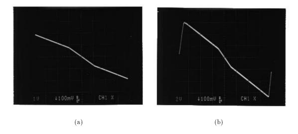
Figure 13: Measured v-i characteristic of negative resistor. (a)  $v_S$  is a triangular waveform with zero dc offset, amplitude 7V peak-to-peak, and frequency 30 Hz. Horizontal axis:  $v_R$  (1V/div); Vertical axis:  $-v_{i_R}$  (100mV/div); (b)  $v_S$  is a triangular waveform with zero dc offset, amplitude 15V peak-to-peak, and frequency 30 Hz. Horizontal axis:  $v_R$  (2V/div); Vertical axis:  $-v_{i_R}$  (100mV/div).
