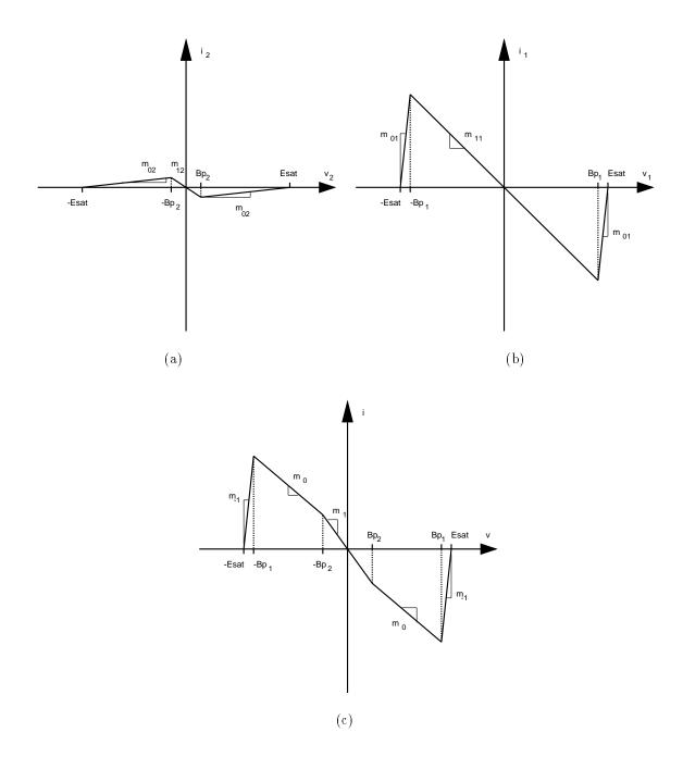
Figure 9: Graphical combination of piecewise-linear voltage-controlled resistors: (a) v-i characteristic of  $N_{R2}$ ; (b) v-i characteristic of  $N_{R1}$ ; (c) v-i characteristic of  $N_{R2}$  in parallel with  $N_{R1}$ .
