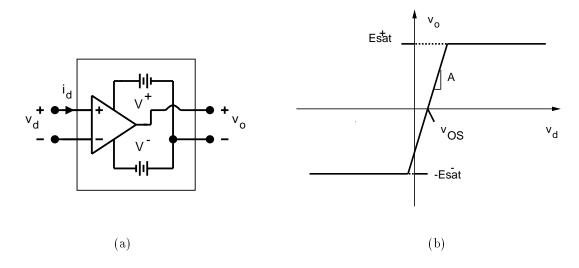
Figure 6: (a) Operational amplifier with associated power supplies; (b) Voltage transfer characteristic of op amp.
