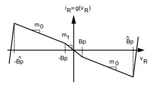
Figure 3: Every physically realizable nonlinear resistor  $N_R$  is eventually passive — the outermost segments (while not necessarily linear as shown here) must lie completely within the first and third quadrants of the v-i plane for sufficiently large |v| and |i|.
