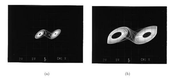
Figure 17: When the attractor is too large, we cannot neglect the effects of the outer regions of the five-segment v-i characteristic. (a)  $C_1 = 10$ nF: Double Scroll attractor is restricted to the regions of negative slope; (b)  $C_1 = 8$ nF: attractor is distorted by the outer positive-going segments.
