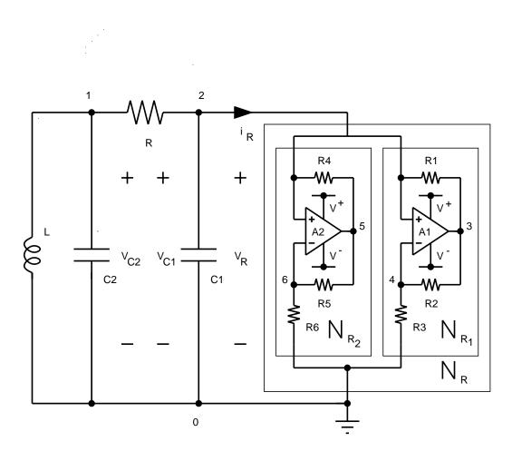
Figure 10: Realization of Chua's circuit using two op amps and six linear resistors to implement  $N_R$ . The two op amps are available in a single eight-pin DIP.
