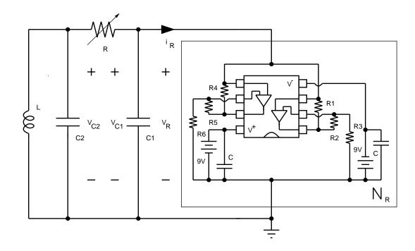
Figure 11: Practical realization of Chua's circuit using an eight-pin dual op amp integrated circuit.
