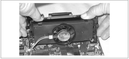
Figure 4-18. Using both thumbs to press firmly until the processor seats fully
