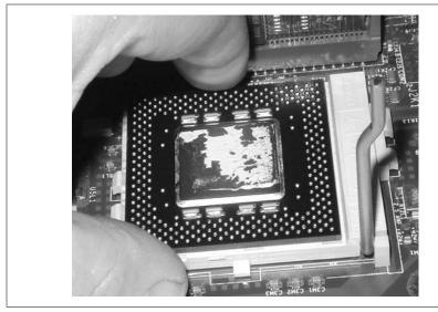
Figure 4-14. Dropping the processor into the socket, where it should seat fully by its own weight (Be sure to align the pins first)
