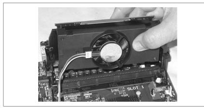
Figure 4-17. Guiding the processor into place, while aligning the keying tab in the slot with that in the processor's card-edge connector
