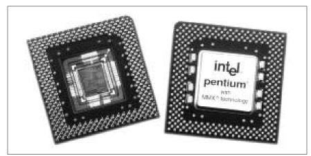
*Figure 4-1. Intel Pentium/MMX processor (photo courtesy of Intel Corporation)*
