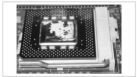
Figure 4-15. The ZIF lever pressed down and locked into place
