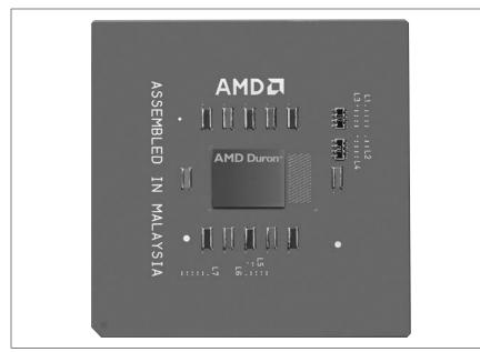
Figure 4-13. AMD Duron processor (image courtesy of Advanced Micro Devices, Inc.)
