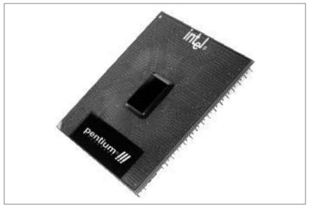
*Figure 4-8. Intel Pentium III processor in FC-PGA package (photo courtesy of Intel Corporation)*
