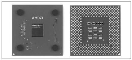
Figure 4-12. AMD Athlon XP processor (image courtesy of Advanced Micro Devices, Inc.)
