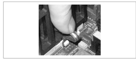
Figure 4-16. Attaching the heatsink securely using the locking clips
