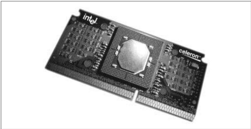
Figure 4-3. Intel Celeron processor in SEPP package (photo courtesy of Intel Corporation)
