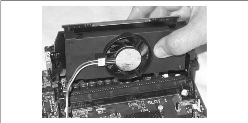
Figure 4-17. Guiding the processor into place, while aligning the keying tab in the slot with that in the processor's card-edge connector
