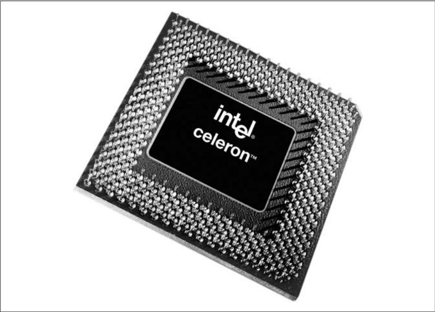
Figure 4-4. Intel Celeron processor in PPGA package (photo courtesy of Intel Corporation)
