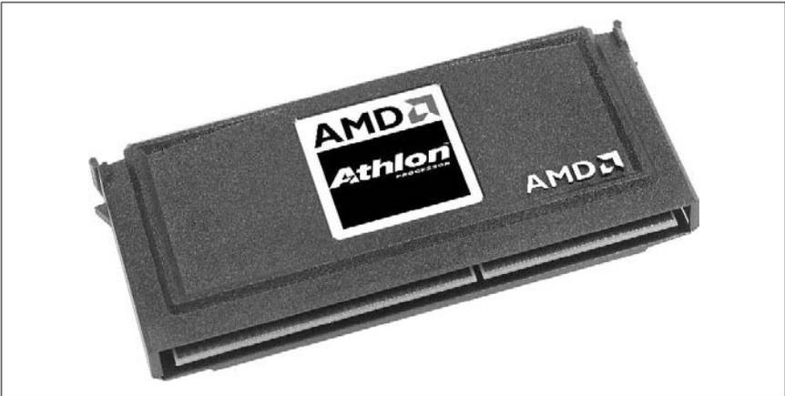
Figure 4-10. AMD Slot A Athlon processor
